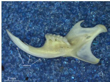
Fig. 2. Precise 150 \mu\text{m} diameter, 1.3 W power 10600 nm laser ablations on modern Mus spretus incisor enamel. \text{CO}_2 produced from 32 consecutive laser shots was collected and analysed for a single carbon and oxygen isotope measurement.
